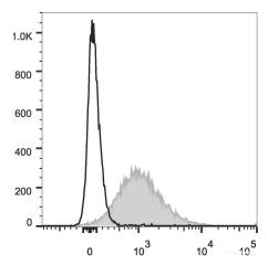
C57BL/6 murine splenocytes are stained with PE/Cyanine5.5 Anti-Mouse CD86 Antibody (filled gray histogram). Unstained splenocytes (empty black histogram) are used as control.
