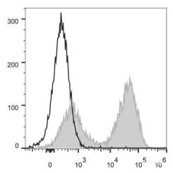
C57BL/6 murine splenocytes are stained with PerCP/Cyanine5.5 Anti-Mouse MHC II (I-A/I-E) Antibody (filled gray histogram). Unstained splenocytes (empty black histogram) are used as control.
